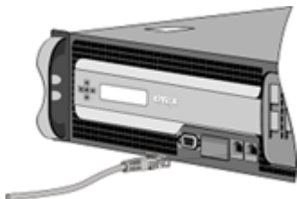
Figure 8. Insert an Ethernet cable
