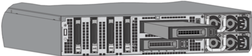
Figure 7. Insert the replacement hard disk drive
