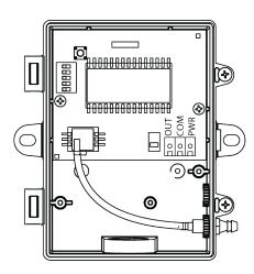
Wiring for output signals and 24 Vac/Vdc power from controller
