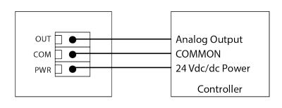
Figure 6a: Wiring (-P models)
