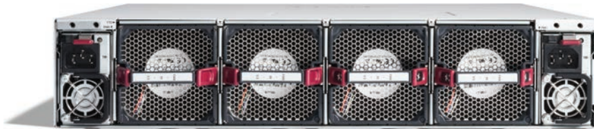
Figure 10-6 A Cisco Systems 8200 Series Router
