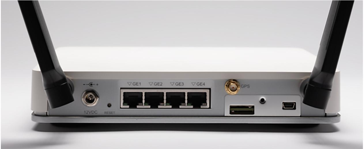
**Figure 1. Connect antennas**
