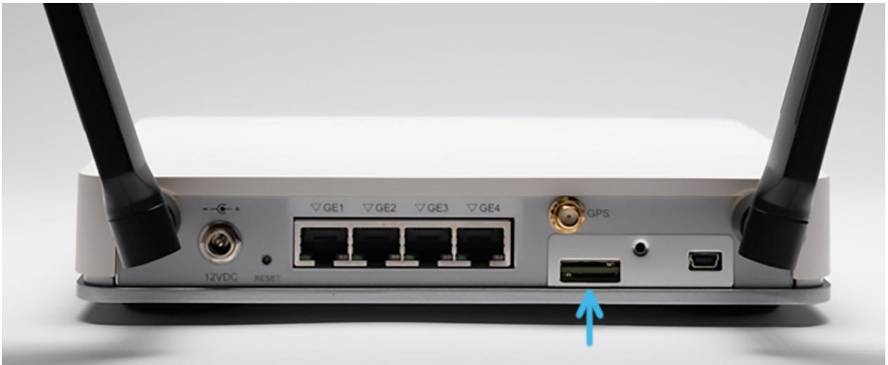
**Figure 2. Insert SIM card**
