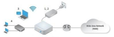
1. Connect the two identical antennas (included in the box) to the MAIN and AUX SMA connectors on the back of the Edge. The GPS antenna (not included) is optional.
