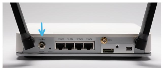
Figure 3. Connect the power adapter to the AC power outlet
