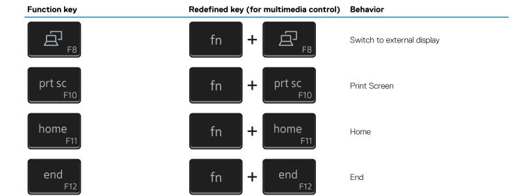
The  ${\bf Fn}$  key is also used with selected keys on the keyboard to invoke other secondary functions.
