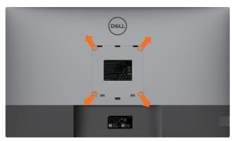
NOTE: Use M6  $\times$  12 mm (200 mm  $\times$  200 mm) or M4  $\times$  12 mm (100 mm  $\times$  100 mm) screws to connect the monitor to the wall-mounting kit.
