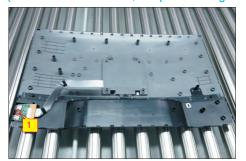
S9 Tear off 1pcs aluminium foil for unfixing the function key cable.
