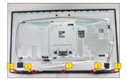
Use a Philips-head screwdriver to remove 2pcs screws(left and right) for unlocking the front bezel with the panel module, then disassemble the front bezel with the unit and put it aside.
