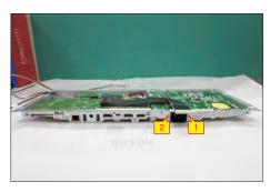
Use a Philips-head screwdriver to remove 7pcs screws for unlocking power board and interface board.
