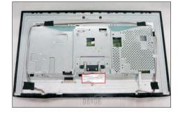
Tear off 2pcs acetate tape for releasing the panel lamp cables. Use a proper tool to release the function key cable from the connector, then pull the function key cable high for releasing the function key cable as the picture below shown.
