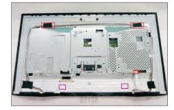
Use a Philips-head screwdriver to remove 5pcs screws for unlocking the front bezel with the assembled unit.
