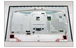
Use a Philips-head screwdriver to remove 4pcs screws for unlocking the bracket chassis module.
