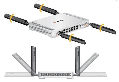
**STEP 2** Adjust the antenna orientation to receive the optimal signal strength in your environment.
