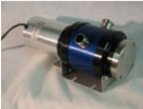
Fig. 6. VAIREX VV-1020 modified vane compressor as delivered.
