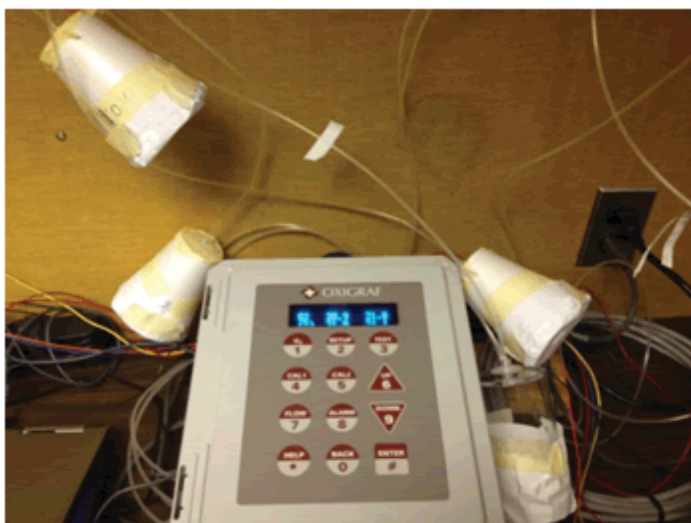
Figure 3. Styrofoam cups that represent the protective metal box used in test bench simulations
