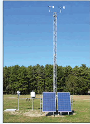
2 & 10 meter tower on the meteorological field
