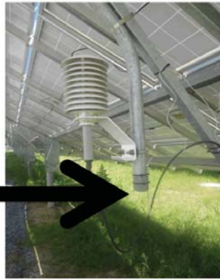
Omega model PRC-10-2-100-1/4-6-e sensor underneath solar panels
