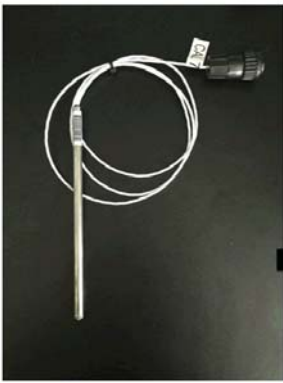
Omega model PRC-10-2-100-1/4-6-e sensor underneath solar panels
