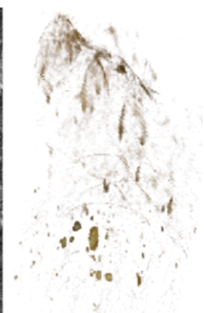
(a) Figure 4: (a) A 2D Image Slice of Mach-1 Catalyst (b) Reconstructed 3D Mach-1 Catalyst
