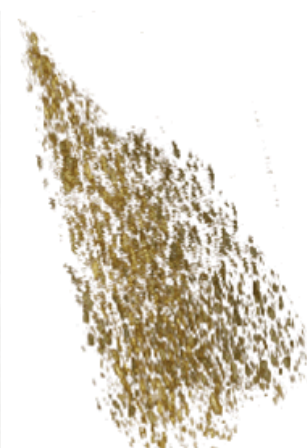
(a) Figure 5: (a) A 2D Image Slice of UCI Catalyst (b) Reconstructed 3D UCI Catalyst
