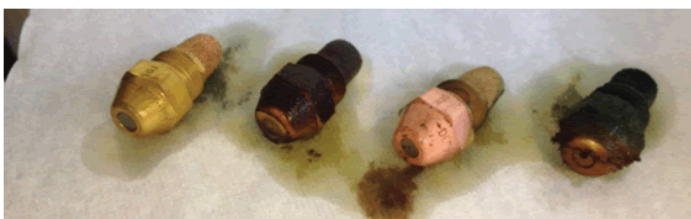
Fig. 6 Yellow metal nozzles post-oven (from left: TAN 0, 2, 4, 20) Source: Andrew Salamone, Michael Worek BNL 2013
