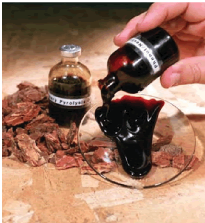
Fig. 1 Non-upgraded pyrolysis oil and wood chips Source: Technical Information Exchange on Pyrolysis Oil 2012
