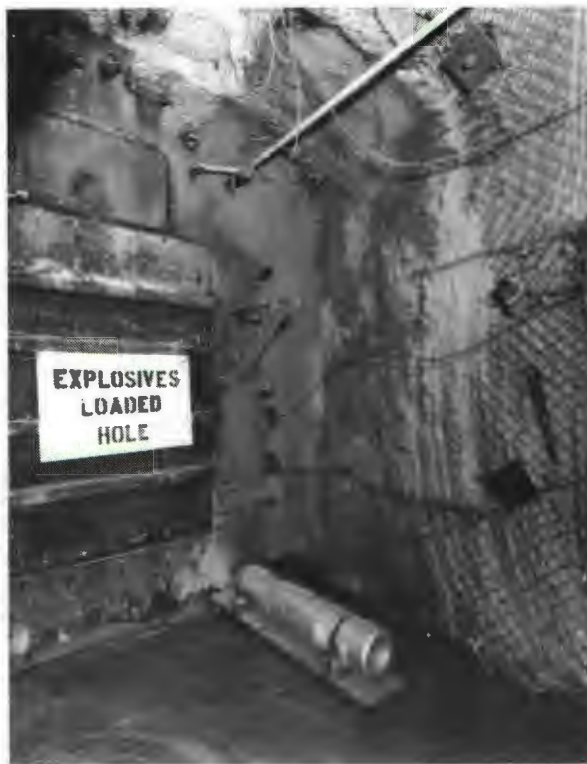
Fig 2. The sulfur hexafluoride bottle was separated from explosion cavity by bulkhead to minimize the possibility for thermal decomposition of tracer gas.
