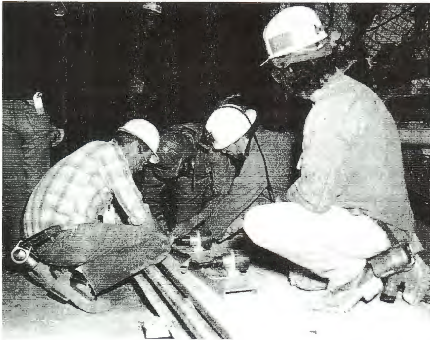
■ Figure 6. Scientists from Los Alamos prepare particle-velocity gages for installation in the rock near the chamber wall.
