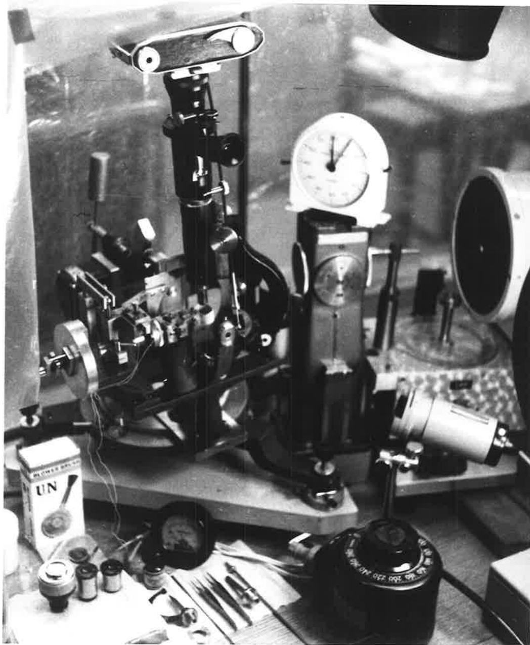
Figure 5(a). The apparatus for combined X-ray diffraction and optical microscopy.
