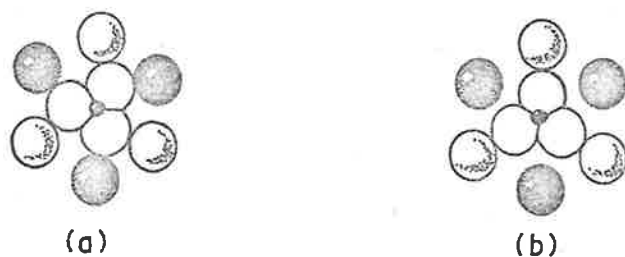
The structure of calcite (a) and aragonite (b), and positions of calcium atoms around the \text{CO}_3^- groups in both structures.
