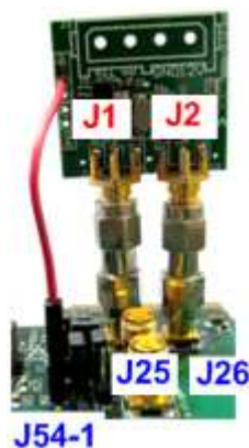
Figure 2-1 Connect CLK SMA board to AC701
