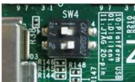
Figure 2-3 SW4 setting to use USB-to-JTAG on ZC706 board
