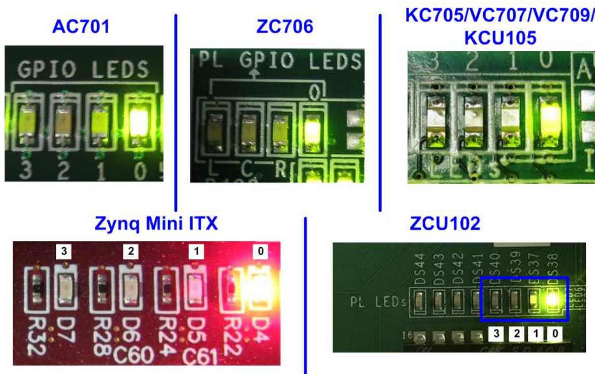
Figure 2-13 LED status after program configuration file and SATA initialization complete
