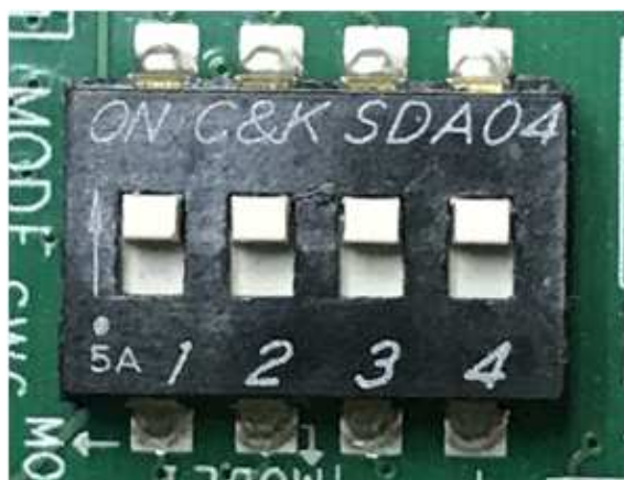
Figure 2-6 SW6 setting to configure PS from JTAG on ZCU102
