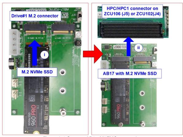
Figure 2-4 Connect AB17-M2FMC connection
