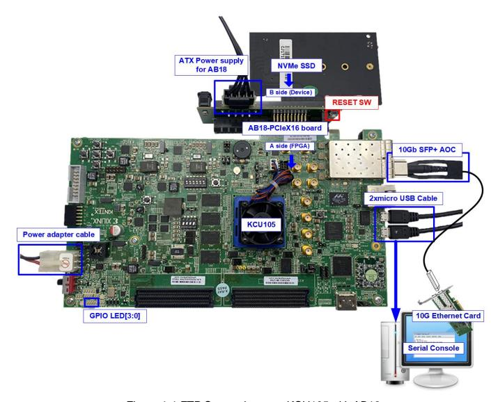
Figure 1-1 FTP Server demo on KCU105 with AB18
