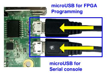
Figure 2-6 micro USB connection of FPGA
