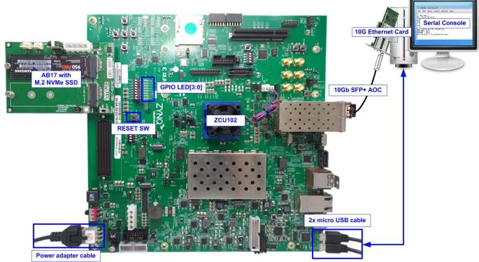
Figure 1-3 FTP Server demo on ZCU102 with AB17
