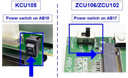
Figure 2-7 Turn on power switch on FPGA and adapter board
