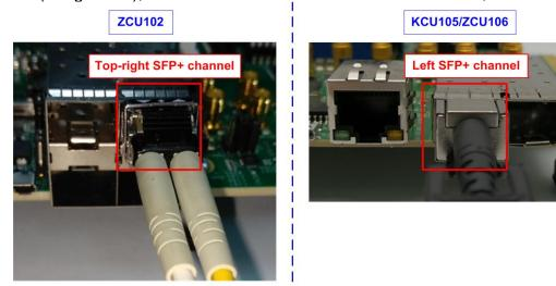
Figure 2-5 SFP+ channel using on ZCU102/ZCU106/KCU105 board
