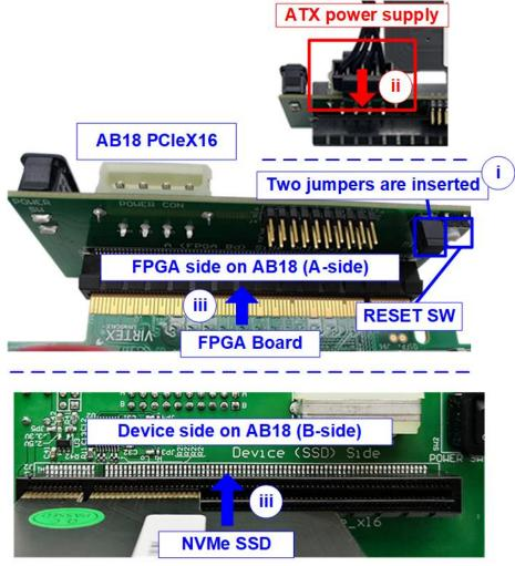
Figure 2-3 Connect AB18-PCIeX16 to KCU105
