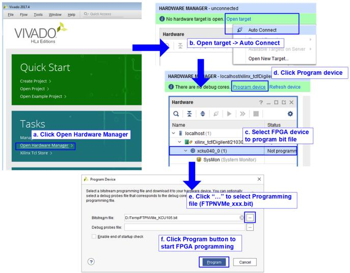
Figure 2-9 Program FPGA by using Vivado
