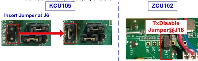
Figure 2-1 Insert jumper to enable SFP+ on KCU105/ZCU102
