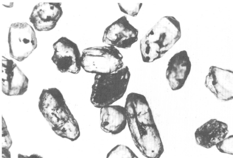
Figure 3. Photomicrograph of zircons from sample 87ANK 081A, fraction ( -150\pm 200 )NMD (table 1). Largest grains are about 150\ \mu\text{m} in length. Note distinct, rounded, dark cores and clear overgrowths on grains.
