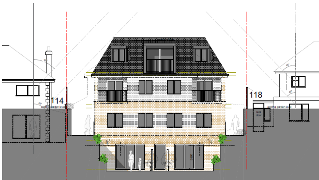
Figure 4: Rear Elevation detailing basement and adjoining occupiers
