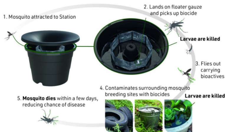
Figure 7. Schematic view of the In2Care Mosquito Trap System.
