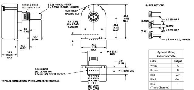
\* Note: For the HEDS-5700, Pin #2 is a No Connect. For the HEDS-5740, Pin #2 is Channel I, the index output.
