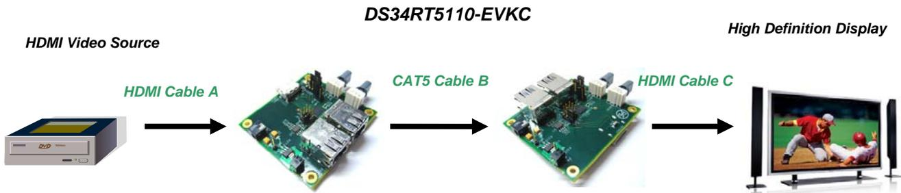
The DS34RT5110 demo kit extends TMDS with the 28 AWG STP DVI cable as follows:
