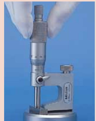
With the disc. anvil (950758) Shown above, the Uni-Mike is used as a height micrometer
