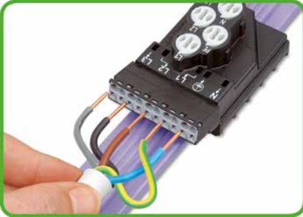
Connecting an installation cable to the supply module. Stripped, solid conductors are simply pushed into unit. Open clamp via screwdriver to insert stripped, fine-stranded conductors.
