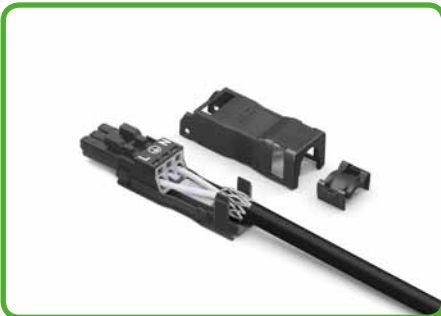
First insert wired connector into strain relief housing, then snap clamp and cover.
