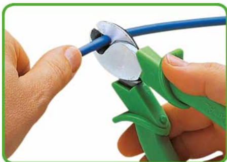
Cutting a cable.
