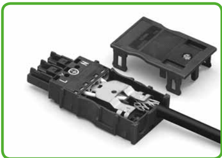
First insert the wired connector into the strain relief housing, then snap the cover and tighten the screw.
