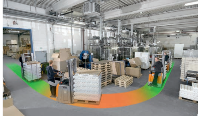
Safe even when cornering: automatic speed reduction around corners
