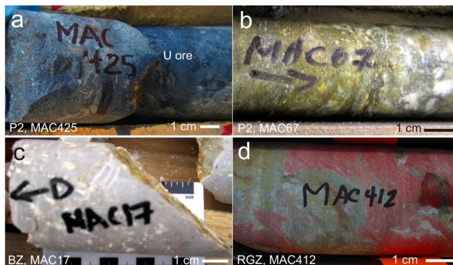
Figure 3.3. Photographs of selected drill-core samples; (a) uranium ore of the Zone 2 ore body and P2 fault (MAC425); (b) intensely sudoite-altered pegmatite from the P2 fault (MAC67); (c) quartzite from the Beached Zone along the unconformity (MAC17); and (d) hematitized and chloritized metapelite from the Red-Green Zone (MAC412). Sample locations are shown in Fig. 3.2.
