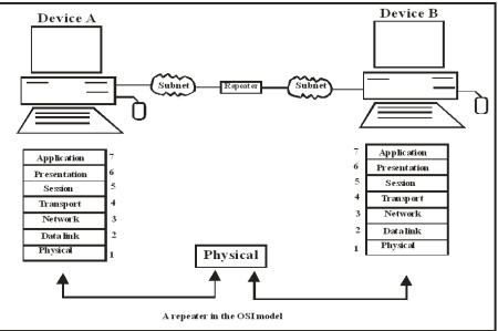
• A repeater allows extending the physical length of a network. The repeater does not change the functionality of the network in any way. The two sections connected by the repeater are in reality one network.
