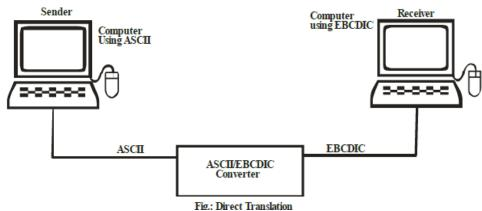
In the given figure ASCII code is transmitted into EBCDIC code at the receiver.
