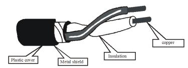
Shielded twisted – pair (STP) cable has a metal foil covering that encases each pair of insulated conductors. This metal casing prevents the penetration of electronic noise.
