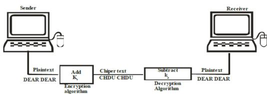
(ii) In poly alphabetic substitution each occurrence of a character can have a different substitute. One possible technique is to find the position of the character in the text and use that value as the key.
