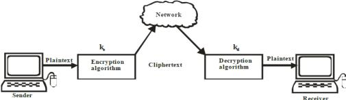
The sender uses an encrypting algorithm and a key to transform the plaintext in to a cipher text. The receiver uses a decryption algorithm and a key transform the cipher text back to the original plaintext.
