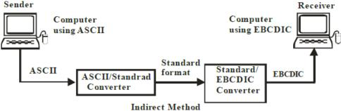
In the given figure ASCII code is translated to a standard format at the sender and translated into EBCDIC at the receiver.
