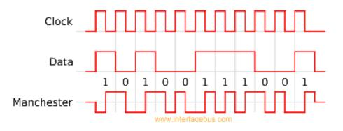
In Manchester encoding, each bit is represented using 2 binary signal voltage levels. Hence,
