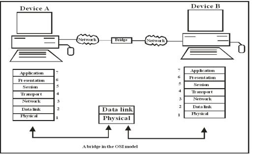
• A bridge operator at the data link layer giving it access to the physical address of all stations connected to it.
