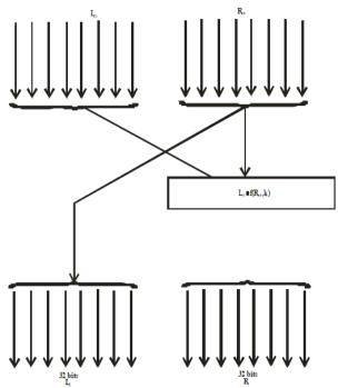
The operation of one of these 16 intermediate stages is illustrated in figure (b). Each stage takes two 32 – bits inputs and produces two 32 – bits outputs. The left output is simply copy of the right input. The right output is the bitwise EXCLUSIVE OR of the left input and a function of the right input and the key for this stage  $K_i$ .
