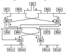
Each bridge identifies a port (the root port) through which it will forward frames to the root bridge. Port conflicts are always resolved in favour of the port with the lower index value. When there is a possibility of multiple bridges forwarding to the same LAN (but not through the root port), ties are broken as follows: bridges closest to the root get preference and between such bridges, the one with the lowest serial number is preferred.
