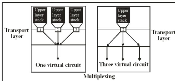
To improve transmission efficiency, the transport layer has the option of multiplexing. Multiplexing at this layer occurs in two ways:
