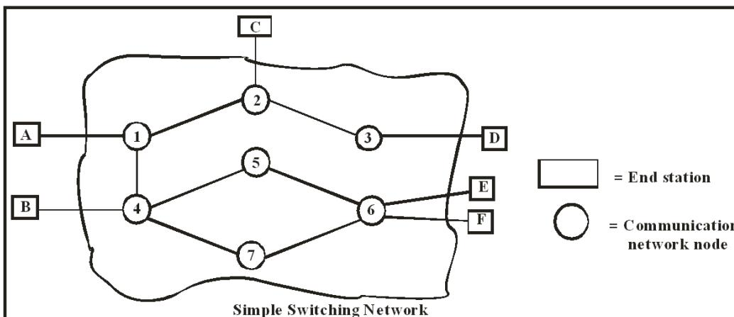
A switching network consists of a series of interlinked nodes, called **switching**. Switching are hardware and/or software devices capable of creating temporary connections between two or more devices linked to the switch but not to each other. In a switched network some of these nodes are connected to the communicating devices, others are used for routing.
