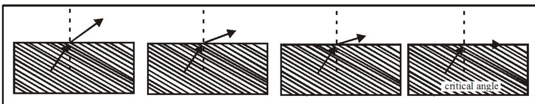
When the angle of incidence becomes greater than the critical angle, the angle of incidence is always equal to the angle of reflection. i.e. when the ray of light reflects off a surface, the angle of incidence is equal to the angle of reflection. Optical fiber is made of glass or plastic and transmits signals in the form of light.
