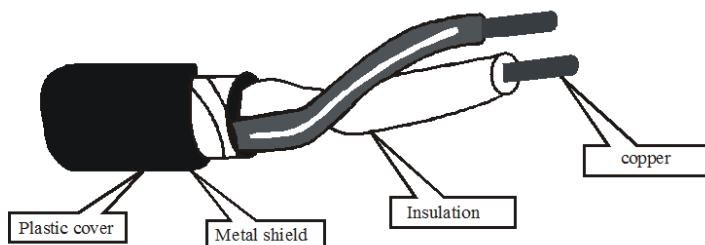
Shielded twisted – pair (STP) cable has a metal foil covering that encases each pair of insulated conductors. This metal casing prevents the penetration of electronic noise.
