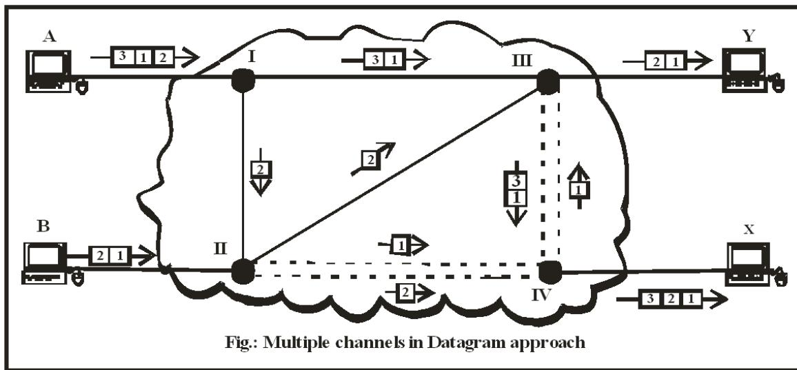
With this approach datagram arrive to their destination out of order. It is the responsibility of the transport layer to reorder the datagram before passing them on to the destination port. The link joining each pair of nodes can contain multiple channels. Each of these channels is capacity is capable of carrying datagram either from several different sources or from one source simultaneously. Packets can be carried simultaneously by either TDM or FDM.
