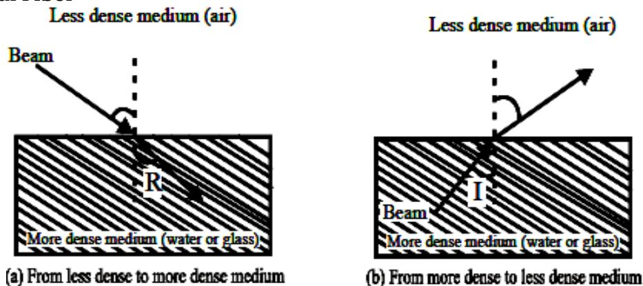
Optical fiber is made of glass or plastic and transmits signals in the form of light. The speed of light depends on the density of the medium through which it is traveling, the higher the density, the slower will be the speed. If a ray of light traveling through one substance suddenly enters into another (less or more dense) substance, its speed changes abruptly, causing the ray to change direction.
