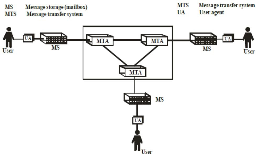
Each user has message storage which consists of disk space in a Mail Storage system and is usually referred to as a mail box. Message storage can be used for storing, sending or receiving messages. The message storage communication with a series of process called **Message transfer agents (MTA)**. The combined MTA make up the message transfer system (MTS).
