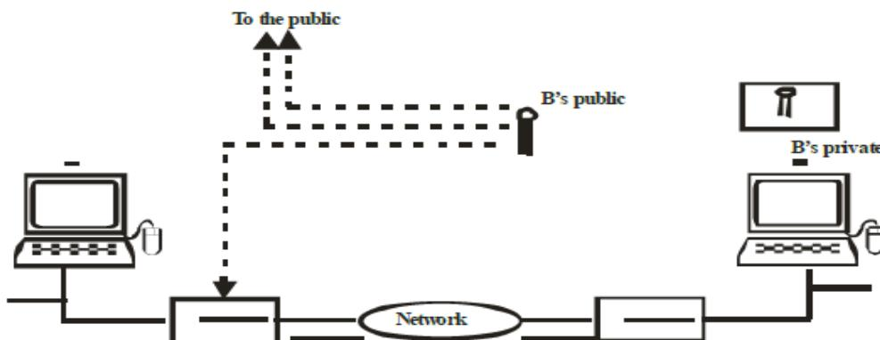
It uses two keys: **a private key and a public key**. The private key is kept by the receiver and public key is announced to the public. The public key that is used to encrypt the algorithm is different from the private key that is used to decrypt the algorithm. The public key is available to the public and the private key is kept by each individual.
