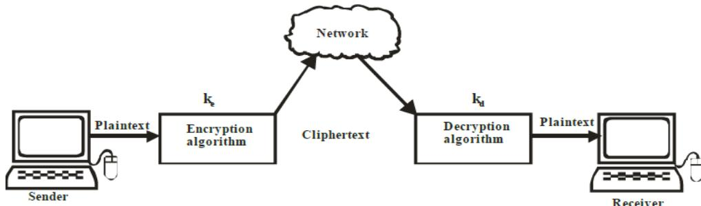
The sender uses an encrypting algorithm and a key to transform the plaintext in to a cipher text. The receiver uses a decrypting algorithm and a key to transform the cipher text back to the original plaintext.
