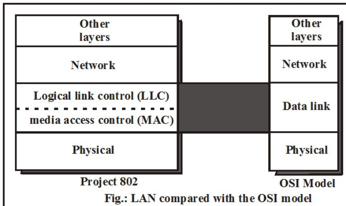
In 1985, the computer society of IEEE developed project 802. It covers the first two layers of the OSI model and part of the third level.
