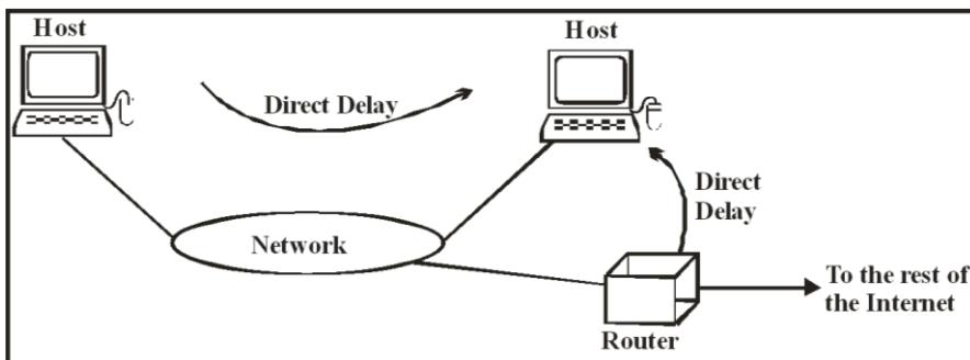
The sender can easily determine if the delivery is direct. It can extract the network address of the destination packet and compare this address of the networks to which it is connected. If a match is found, the delivery is direct.
