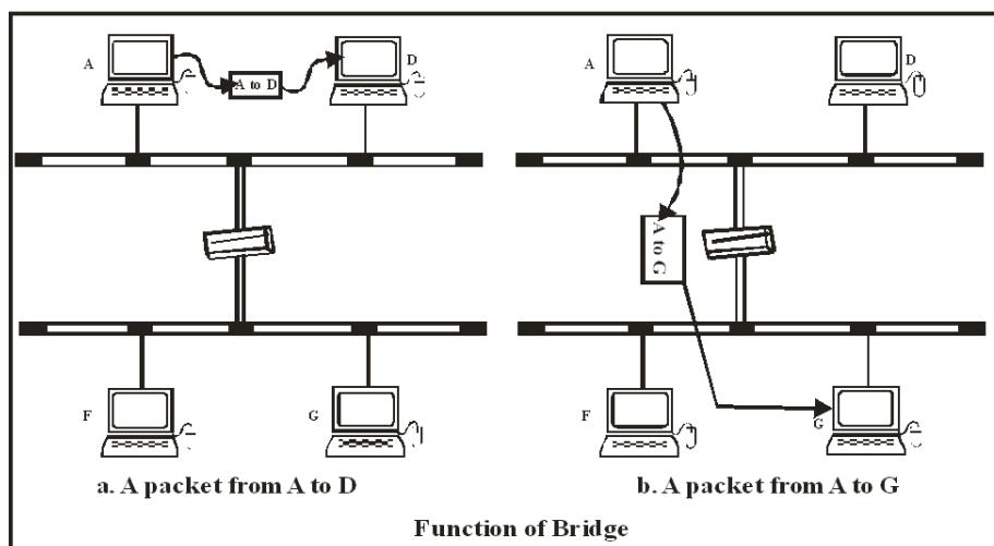
As shown a packet from station A addressed to station D arrives at the bridge. Station A is on the same segment as station D, therefore the packet is relayed to the upper segment and received by station D. In second part, a packet generated by station A is intended for station G. The bridge allows the packet to cross and relays it to the lower segment, where it is received by station G.
