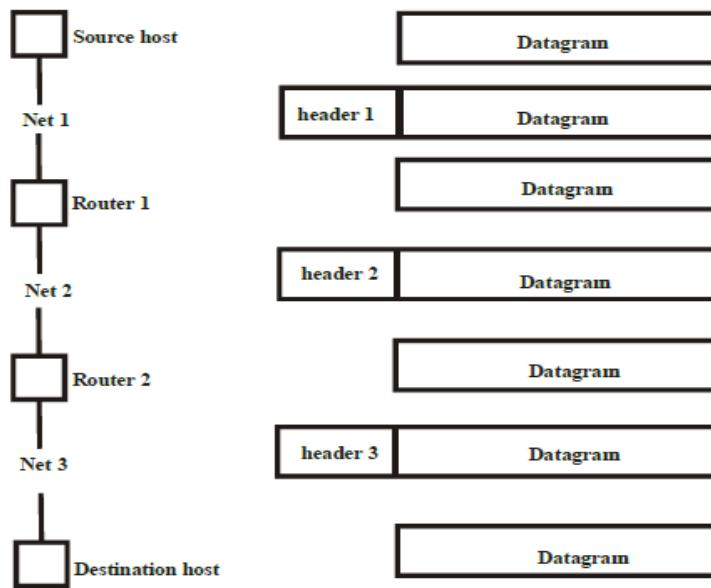
A datagram can travel through different networks. When the frame reaches the next hop, the receiving software removes the IP datagram and discards the frame. If the datagram is to be forwarded across another network, a new frame is created.
