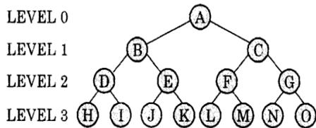
Forward packet to the router at Level 3: Total 6 hops are required if A wants to communicate with any level 3 node. Similarly, 5 hops are required if H wants to communicate with any level 2 node, 4 hops are required if H wants to communicate with any level 1 node and 3 hops are required if H wants to communicate with any level 0 node.
