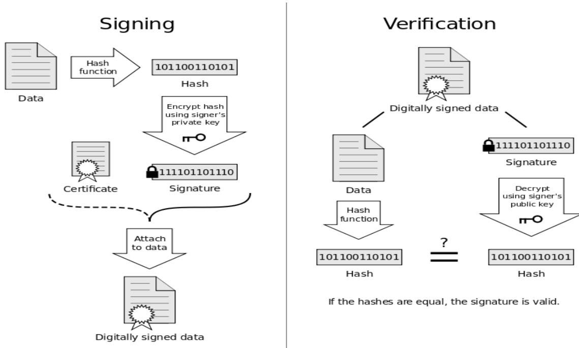
A digital signature scheme typically consists of 3 algorithms;
