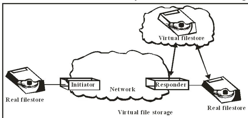
FTAM is based on asymmetrical access of a virtual file. Each transaction requires an initiator and a responder. The initiator request the transfer of access to or management of a file from responder. The responder creates a virtual file model of its actual file allows the initiator to use virtual model rather than the real file. Because the model is software, it can be designed to be independent of hardware and the operating system constraints.
