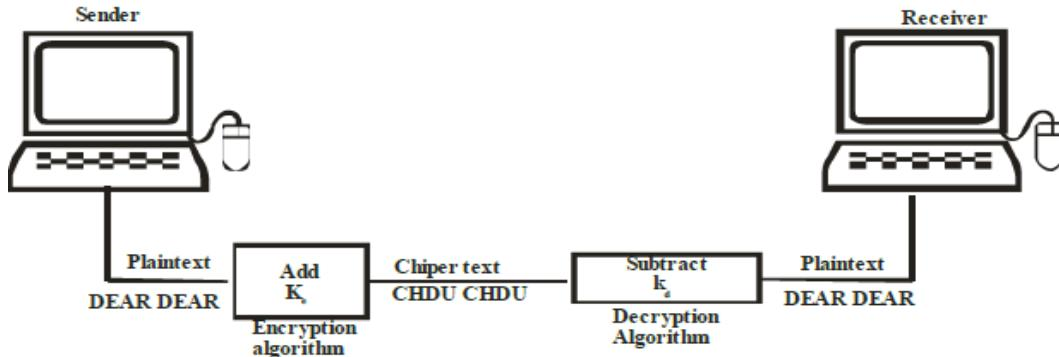
(ii) In poly alphabetic substitution each occurrence of a character can have a different substitute. One possible technique is to find the position of the character in the text and use that value as the key.
