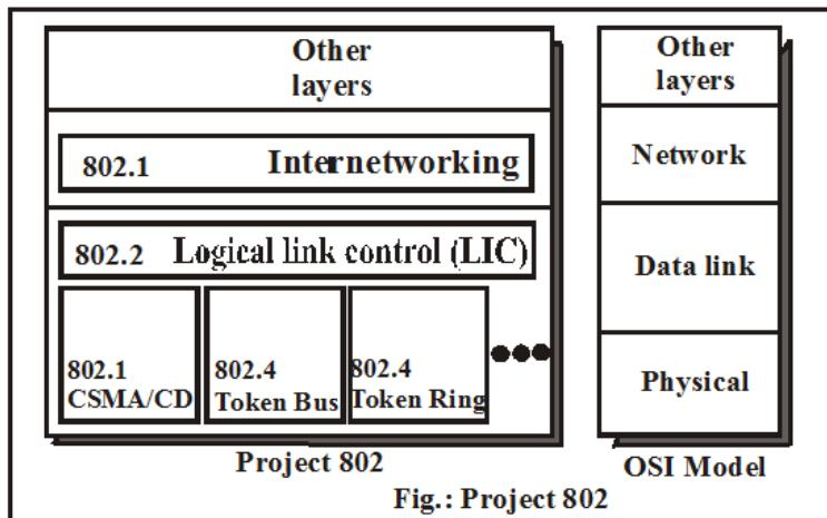
The IEEE project 802 model takes the structure of HDLC frame and divides it into 2 sets of function.
