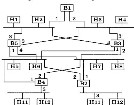
Each bridge identifies a port (the root port) through which it will forward frames to the root bridge. Port conflicts are always resolved in favour of the port with the lower index value. When there is a possibility of multiple bridges forwarding to the same LAN (but not through the root port), ties are broken as follows: bridges closest to the root get preference and between such bridges, the one with the lowest serial number is preferred.
