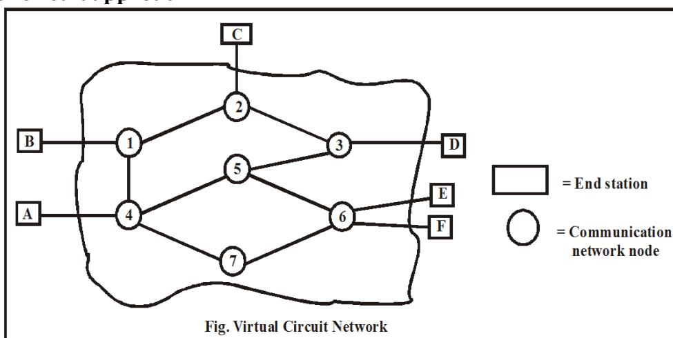
In virtual circuit approach, a route established before are sent. This does not mean that there is a dedicated path as in circuit switching. A packet is still buffered at each node and queued for output over a line.
