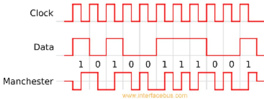
In Manchester encoding, each bit is represented using 2 binary signal voltage levels. Hence,
