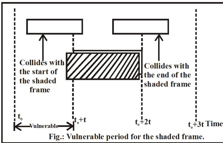
Let  $t$  be the time required to send a frame. If any other user has generated a frame between time  $t_0$  and  $t_0 + t$ , the end of that frame will collide with the shaded one. Similarly any other frame started between  $t_0 + t$  and  $t_0 + 2t$  will collide with the end of the shaded one. If the frame starts after  $t_0 + 2t$  time, there given by Poisson distribution
