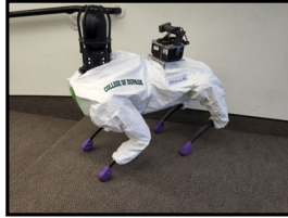
Spot at a Fermi Lab demonstration wearing its PPE. A radiation sensor and other equipment attached
