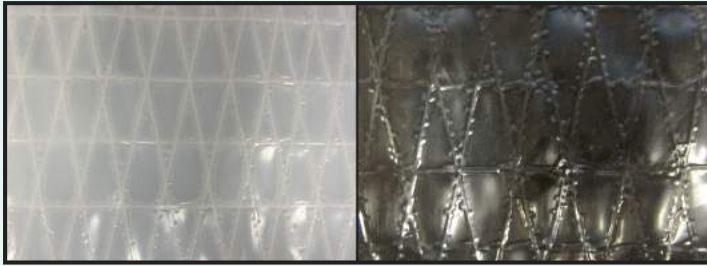
Detail of reinforced string tarps
