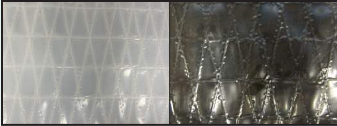
Detail of reinforced string tarps
