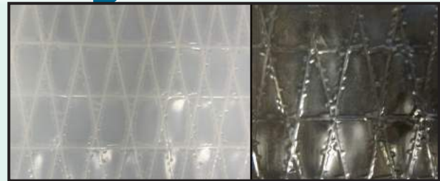
Detail of reinforced string tarps
