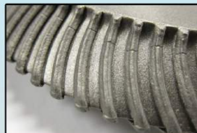
Disc wear after 190,000 tons of silage
