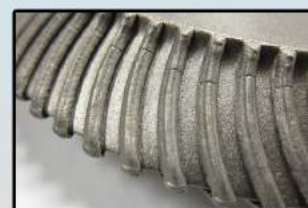
Disc wear after 190,000 tons of silage
