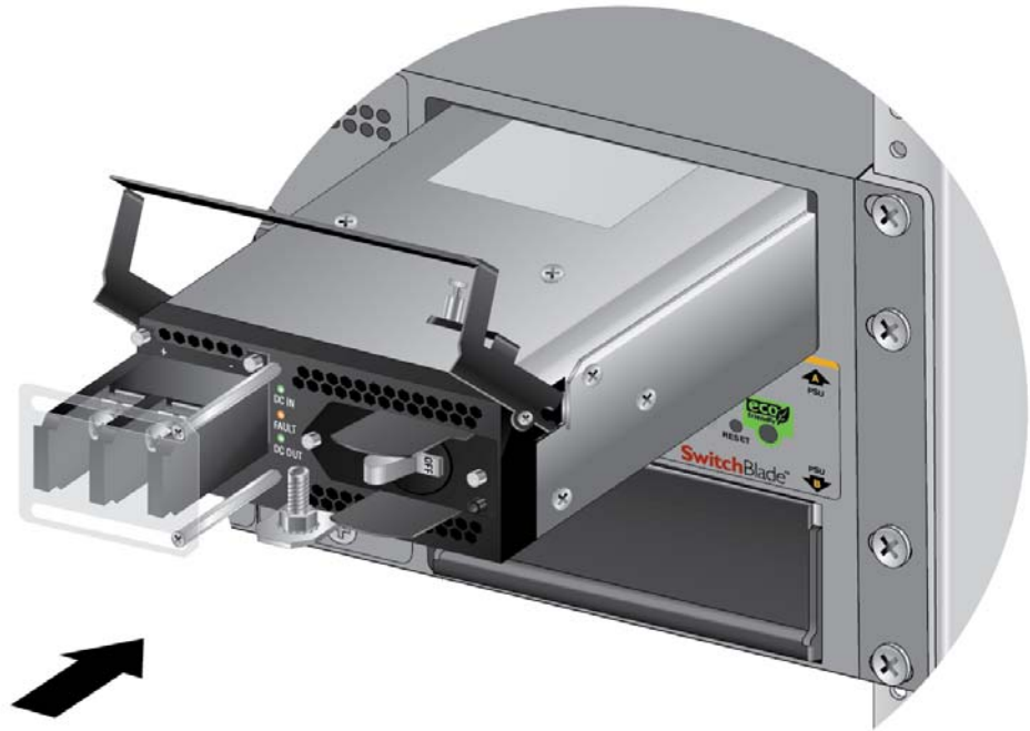
Figure 40. Inserting the SBxPWRSYS1-80 DC Power Supply
