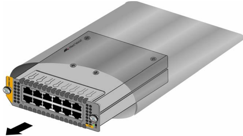
Figure 43. Removing the Ethernet Line Card from the Anti-static Bag
