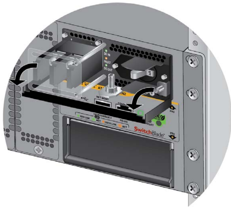
Figure 41. Lowering the Locking Handle on the SBxPWRSYS1-80 DC Power Supply
