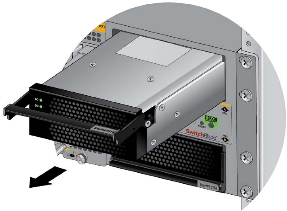
Figure 106. Removing the SBxPWRSYS2 AC Power Supply
