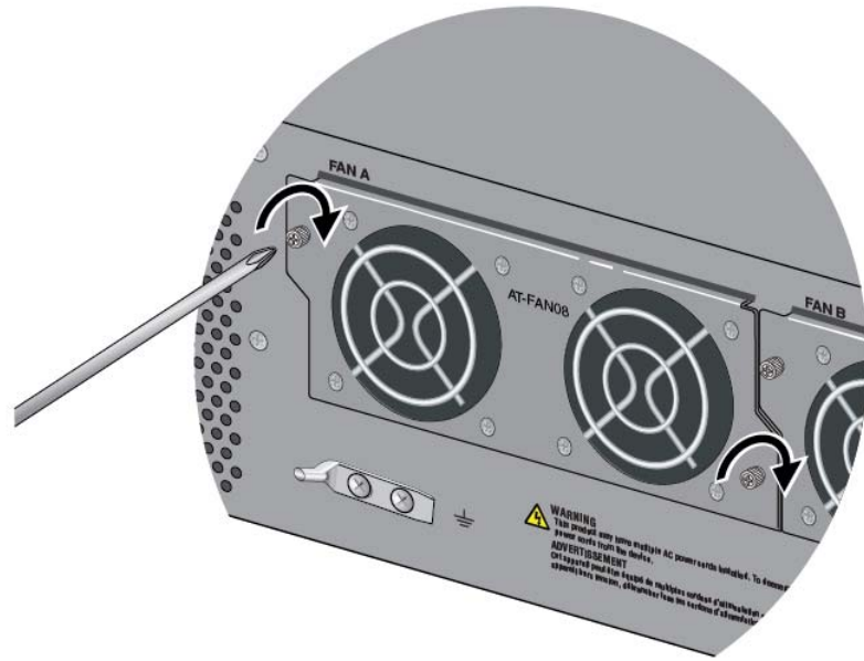
Figure 126. Tightening the Two Captive Screws on the FAN08 Module
