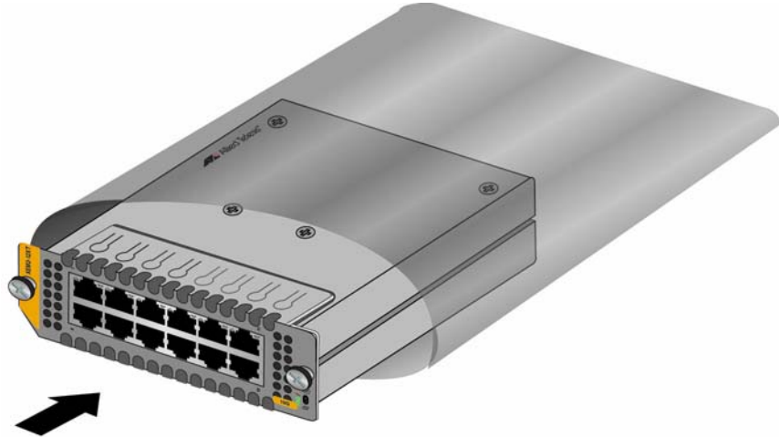
Figure 121. Placing the Ethernet Line Card in its Anti-static Bag
