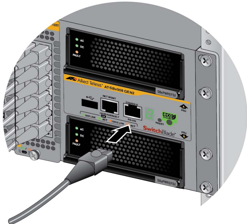
Figure 88. Connecting the Management Cable to the Console RS-232 Port
