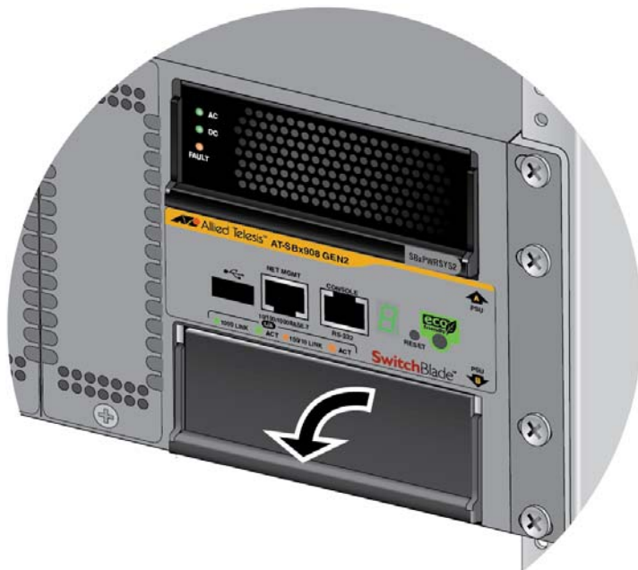
Figure 51. Lowering the Locking Handle on the Blank Power Supply Slot Cover
