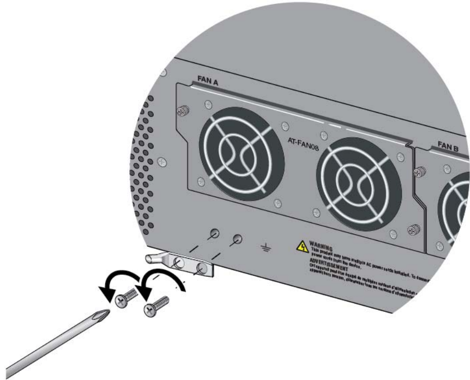
Figure 30. Removing the Grounding Lug from the Chassis
