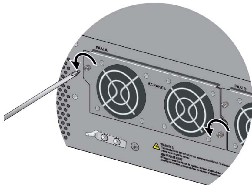
Figure 122. Loosening the Screws on the FAN08 Module
