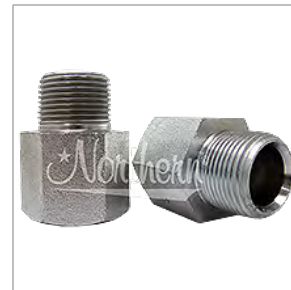
RW8047 (Northern RW8047) ADAPTERS-3/4 NPT MALE X 1-1/16-16 UNF ORING-PAIR
