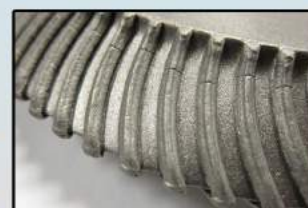
Disc wear after 190,000 tons of silage
