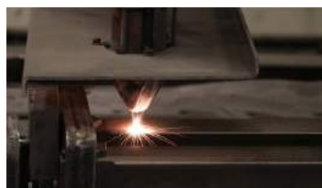
Laser Metal Deposition
