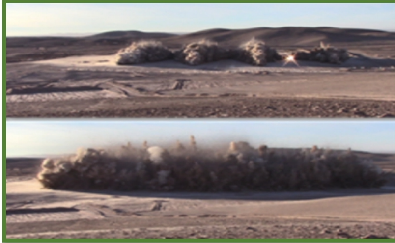
Figure 13-5. Typical Blast in Nueva Victoria Mine (caliches)
