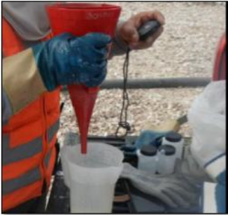
c) Viscosity measurement.
