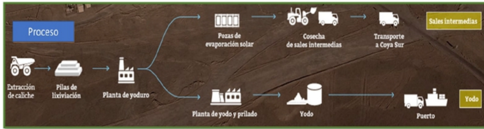
Figure 15-3. Nueva Victoria Plant Process Diagram
