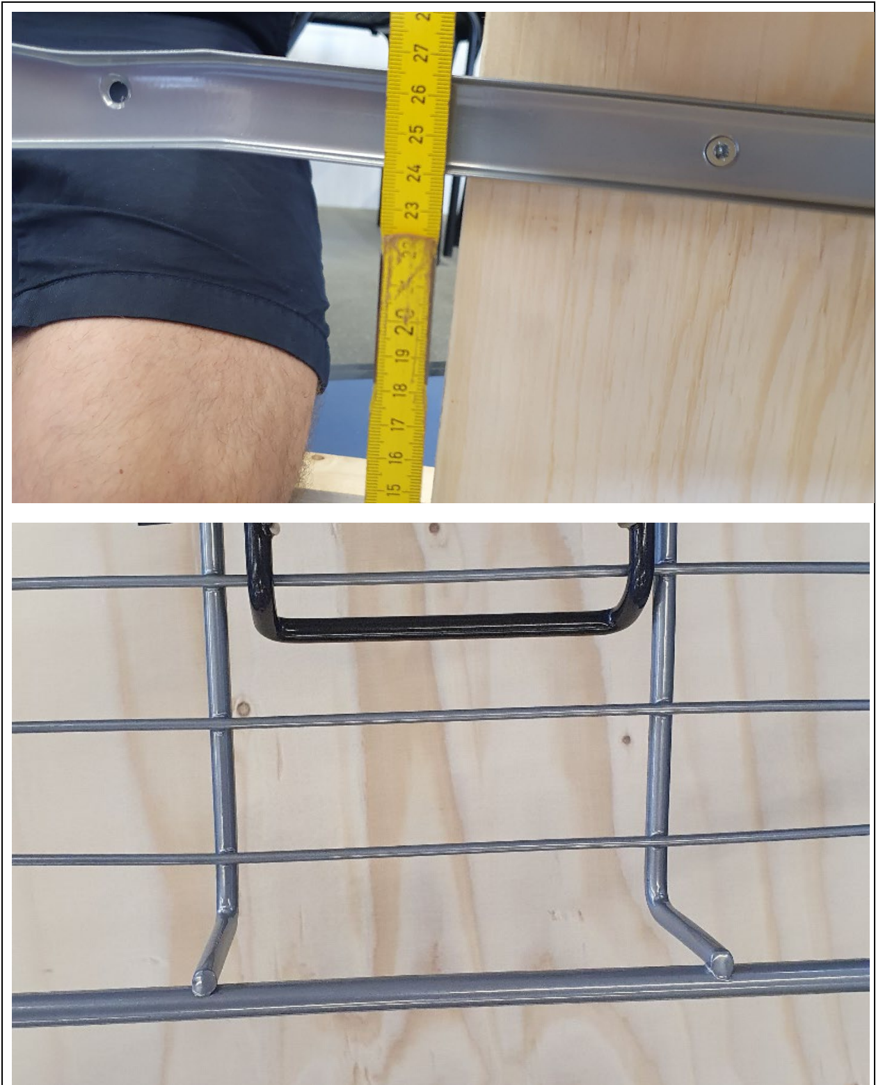
The IKEA products Utrusta and Rinnig have to be mounted such that the lowest Utrusta wire is 150mm above the wooden board (inner height). The plate holder
