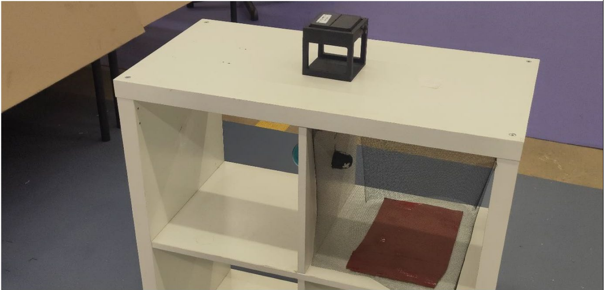
Kallax with space for electronics behind non-transparent curtain and holder for wooden plate on top. (In this figure the curtain is illustrated transparent to show the inside of the shelf)
