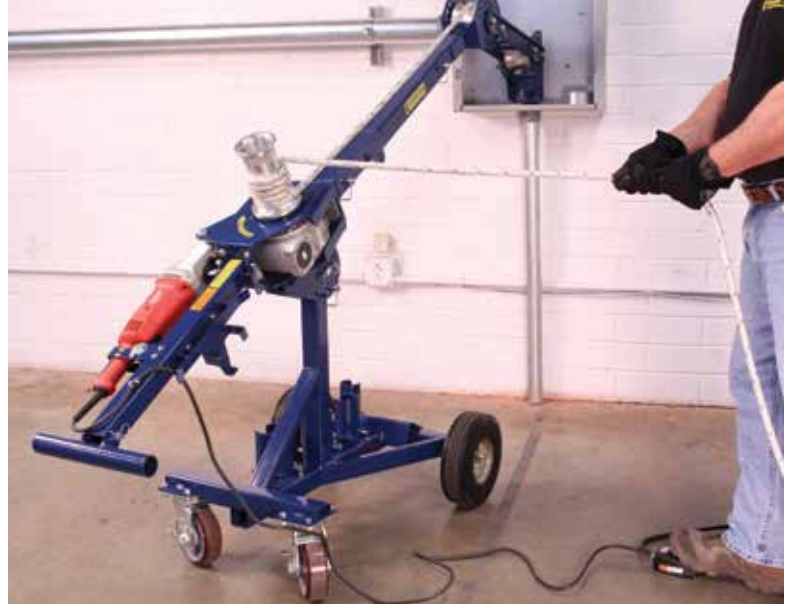
Mobile Cable Puller 6,000 lb. Capacity in use
