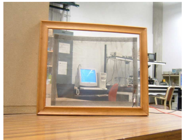
Fig. 5. Photograph of the fabricated film speaker.
