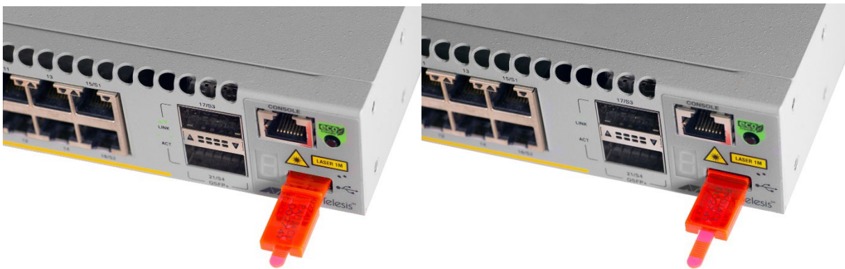
Figure 47: The Difference Between a Partly and Fully Inserted Housing Over Tab
