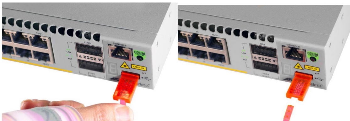
Figure 48: Breaking the Tab on USB Port Lock
