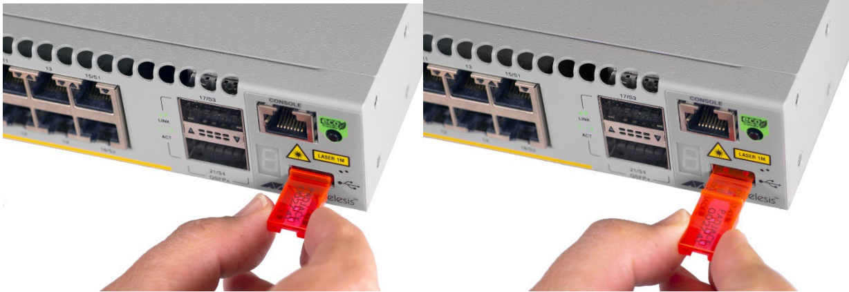
Figure 49: Removing the Housing from USB Port Lock
