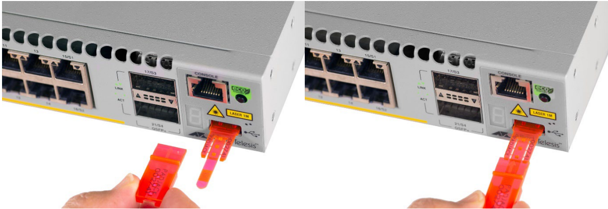
Figure 46: Sliding the Housing Over USB Port Lock Tab
