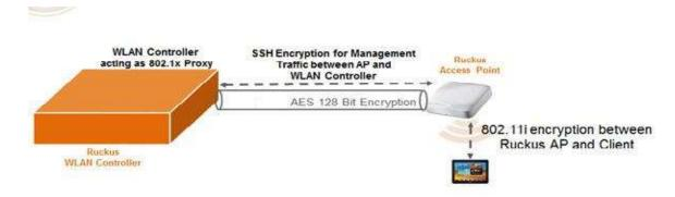
Figure 1: Encryption between AP and Controller
