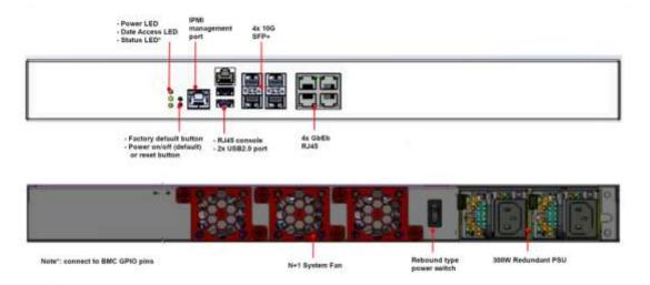
Figure 2: SmartZone 144 Front and Rear View
