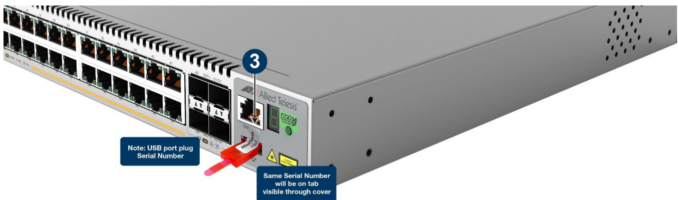
Figure 77: Location of USB Port Plug for x530L-52GTX
