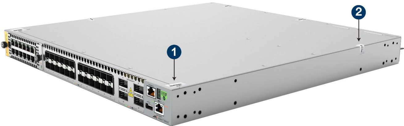
Figure 55: Tamper-Evident Seals on Top Right Side
