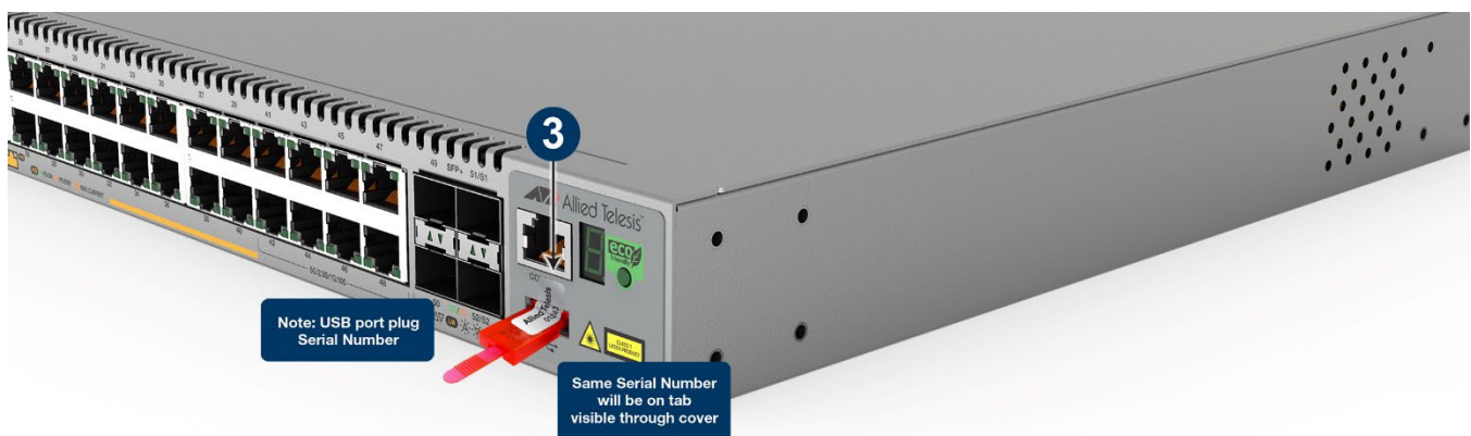
Figure 69: Location of USB Port Plug for x530-52GTXm
