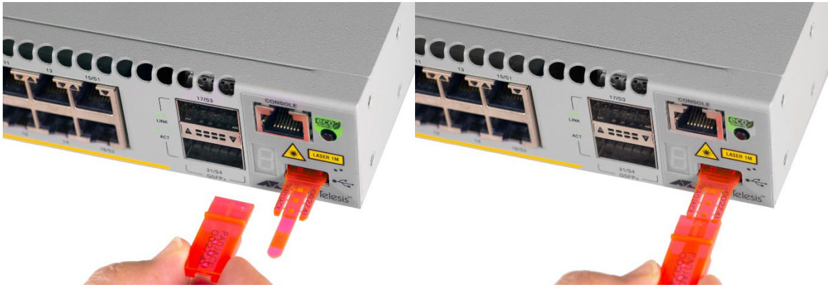
Figure 86: Sliding the Housing Over USB Port Lock Tab
