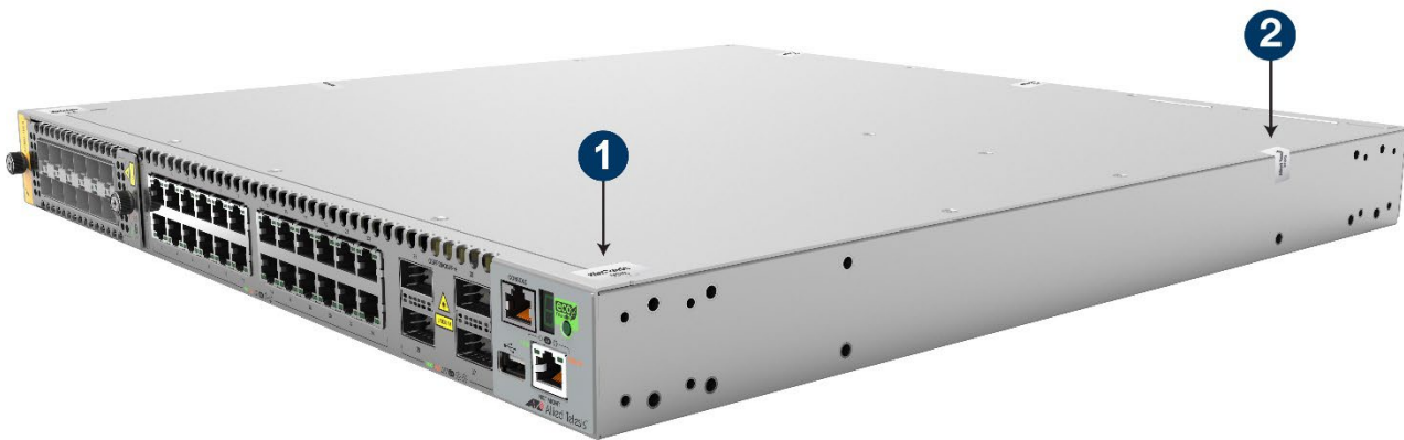
Figure 48: Tamper-Evident Seals on Top Right Side
