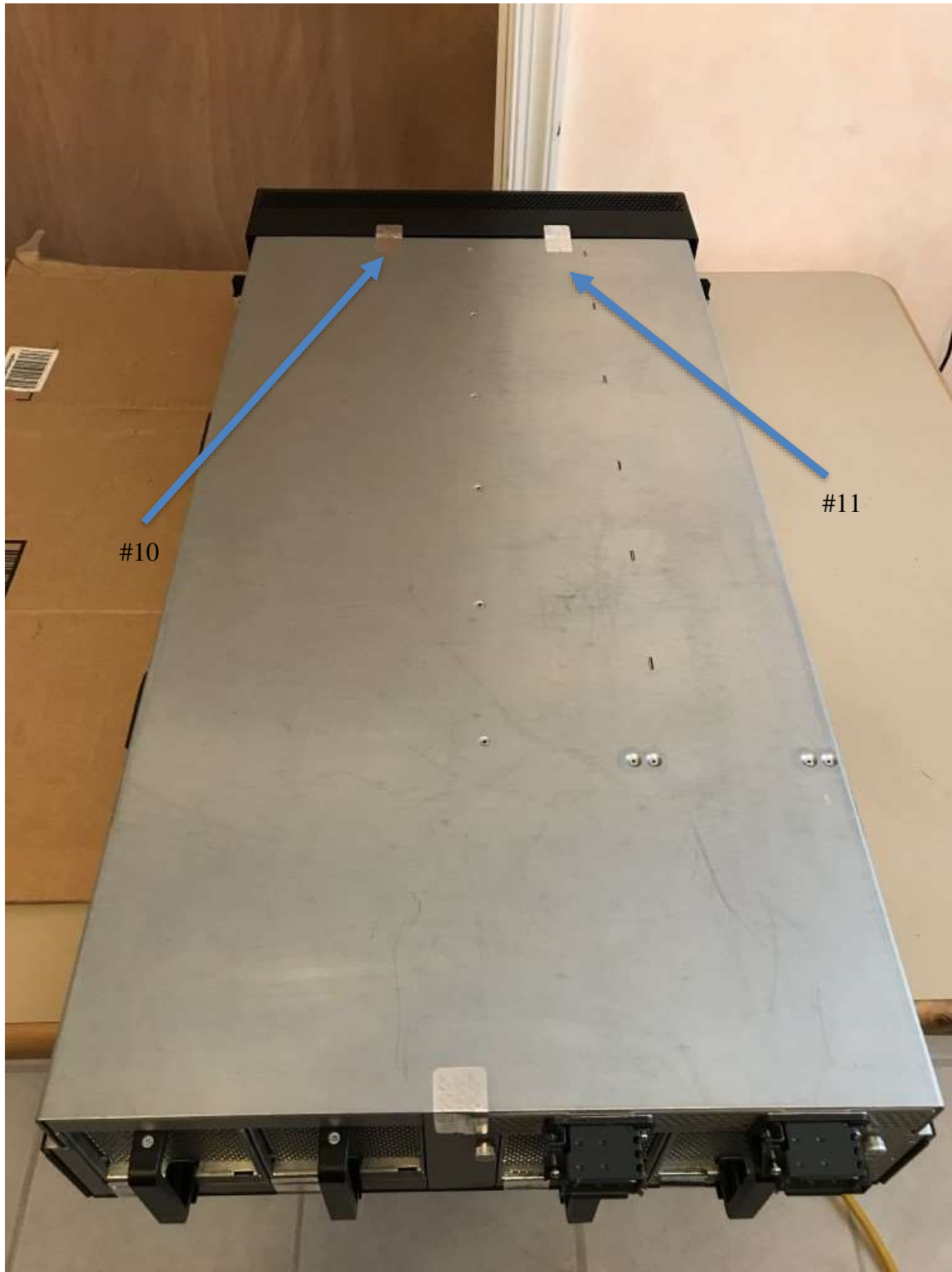
Figure 15: FPR9300 Bottom view (Bottom has TEL #10 and #11 overlapping opacity shield and bottom of chassis, also present is TEL #7 overlapping bottom and back of plug-in)
