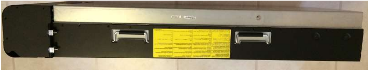
Figure 12: FPR9300 Left view (Left side has no TELs)
