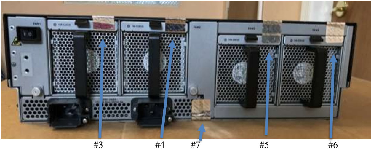
Figure 13: FPR9300 Rear view (Rear has TEL #3, #4, #5, #6, each overlapping chassis and plug-in and #7 on bottom)
