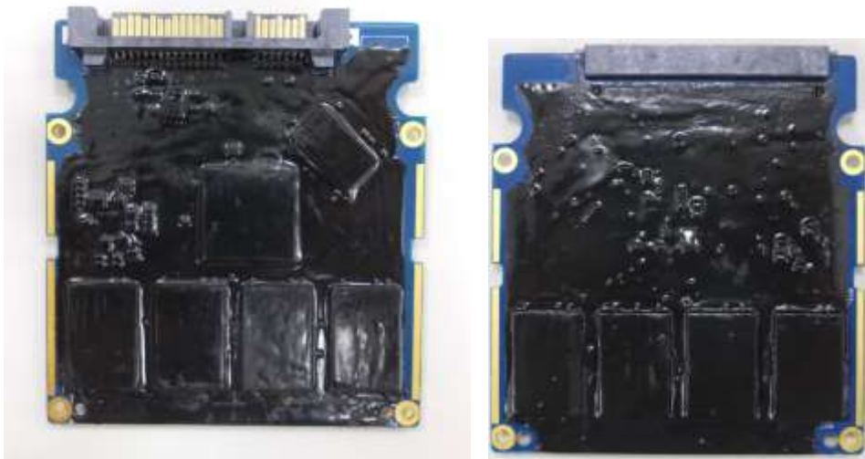
Exhibit 2 - Specification of the PS3112-S12 2.5-INCH SATA NAND FLASH SSD Series Cryptographic Boundary (From left to right: top side, bottom side).
