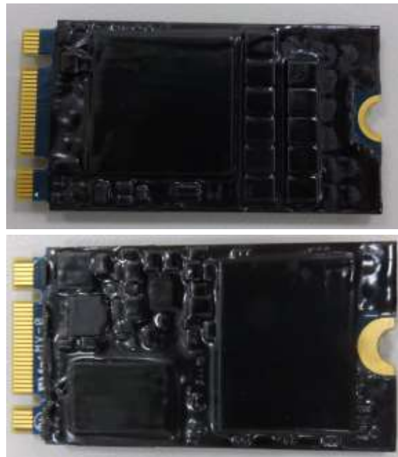
Exhibit 5 - Specification of the PS3112-S12 M.2 2242 SATA NAND FLASH SSD Series Cryptographic Boundary (From top to bottom: top side, bottom side).
