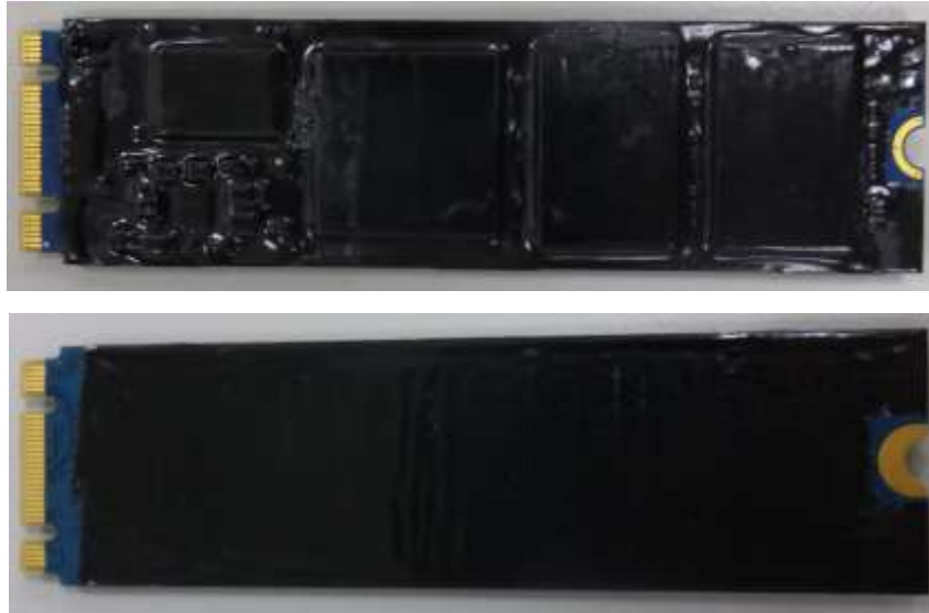
Exhibit 4 - Specification of the PS3112-S12 M.2 2280 SATA NAND FLASH SSD (S3) Series Cryptographic Boundary (From top to bottom: top side, bottom side).
