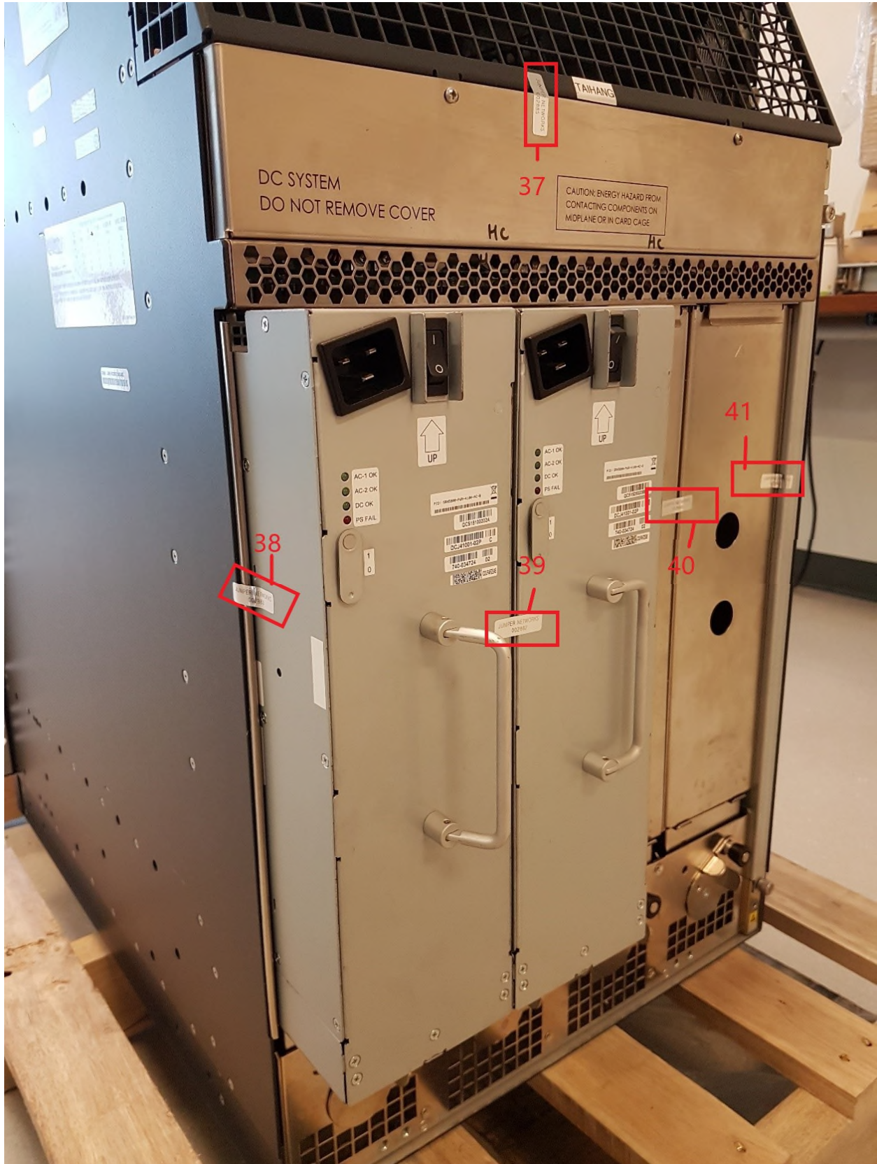
Figure 35 - SRX5800 Tamper-Evident Seal Locations (Rear, five (5) Seals: TEL 37-41)
