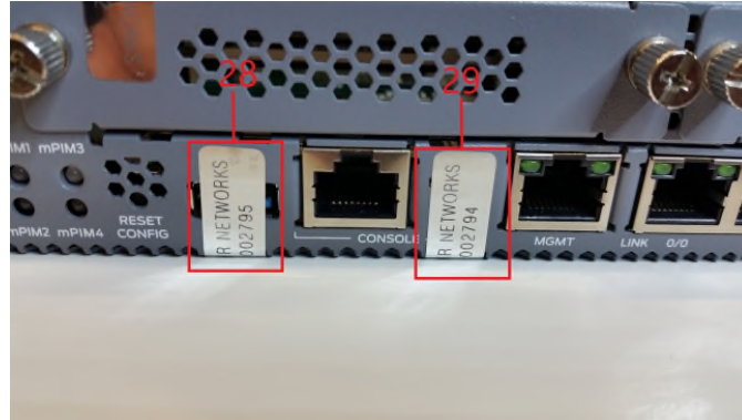
Figure 25 – SRX340/SRX345 Tamper-Evident Seal Placement (USB Ports, Two (2) Seals: TEL 28 & 29)
