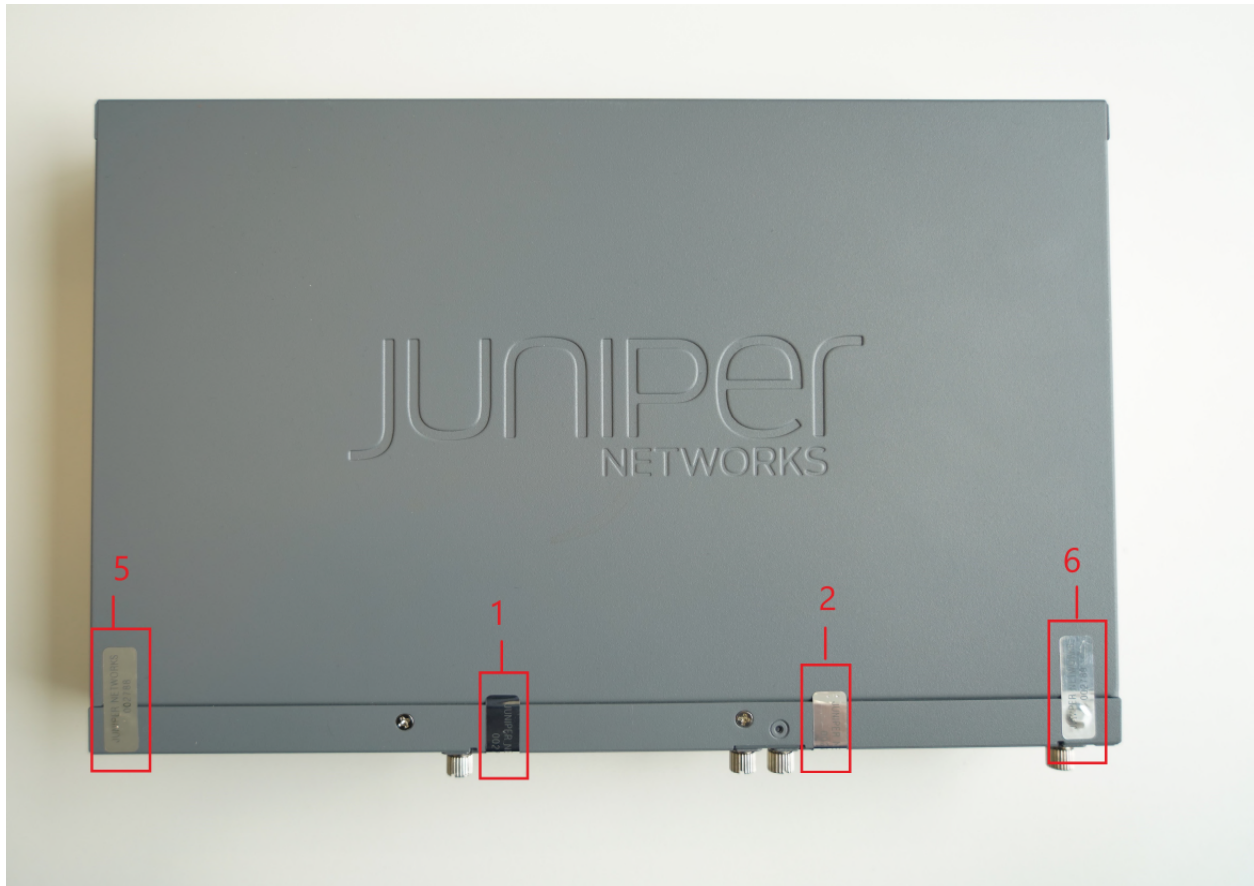
Figure 20 - SRX320 Tamper-Evident Seal Placement (Top Cover Screws (2) Seals TEL 5 & 6)
