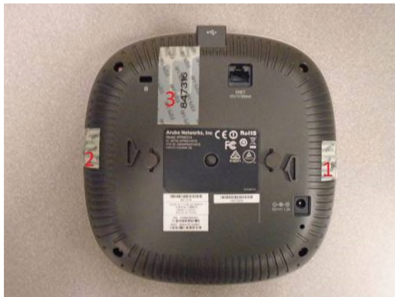
Figure 19 – Bottom View of AP-314 with TELs
