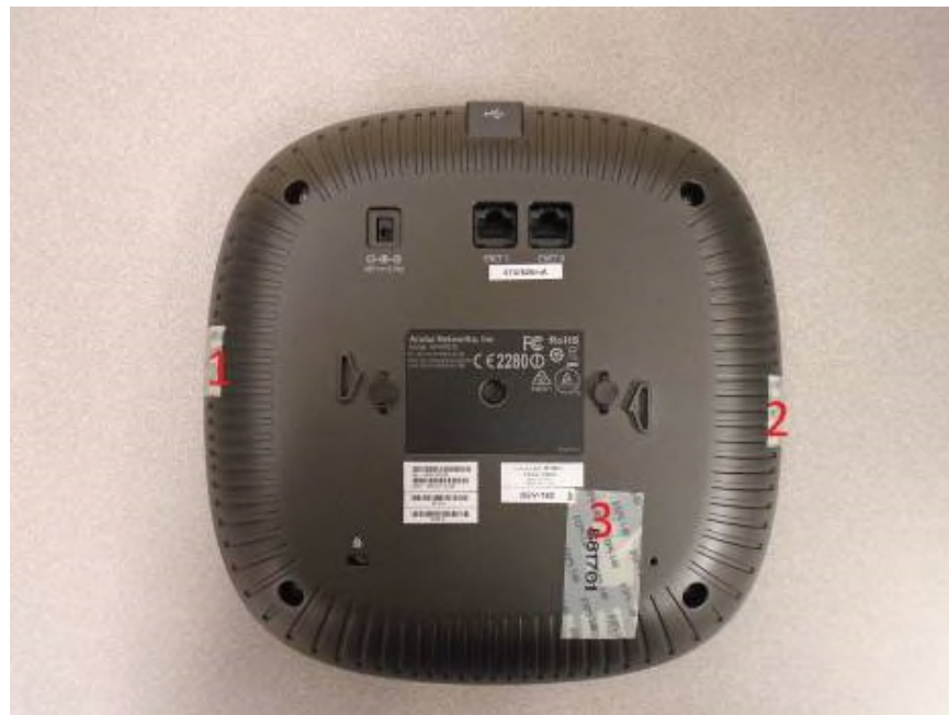
Figure 23 – Bottom View of AP-334 with TELs
