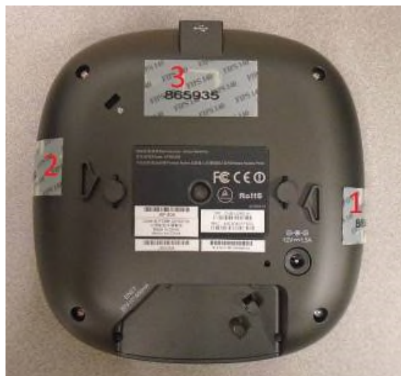
Figure 15 – Bottom View of AP-304 with TELs
