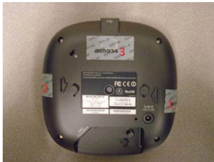
Figure 17 – Bottom View of AP-305 with TELs
