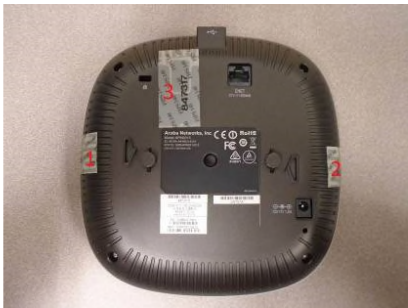
Figure 21 – Bottom View of AP-315 with TELs
