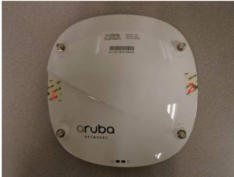
Figure 18 – Top View of AP-314 with TELs
