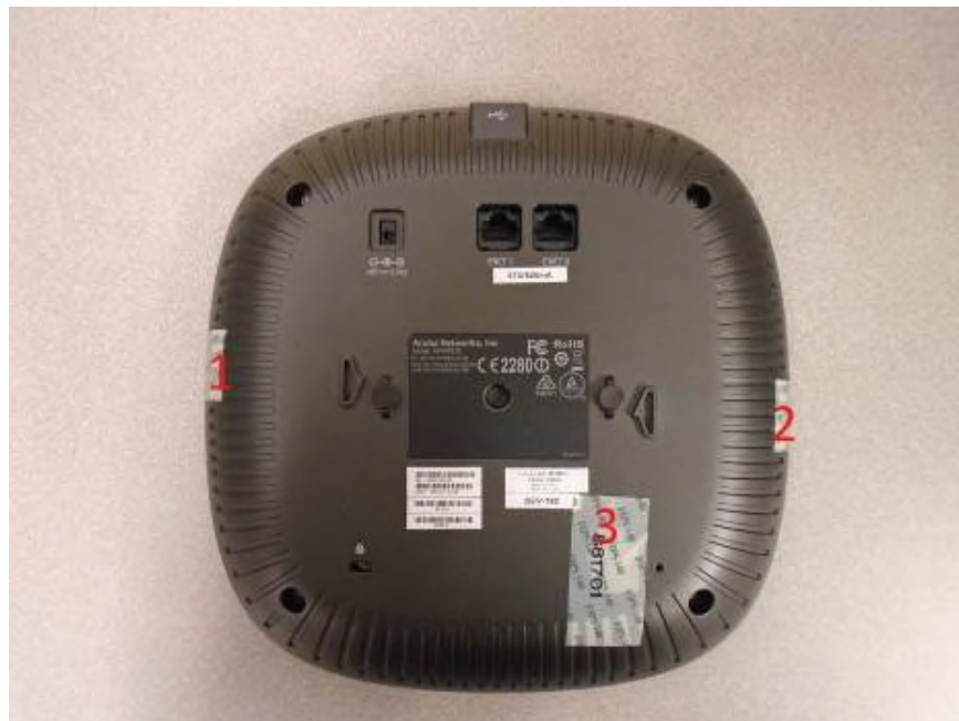
Figure 25 – Bottom View of AP-335 with TELs
