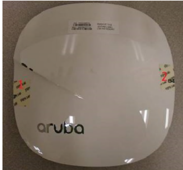
Figure 16 – Top View of AP-305 with TELs
