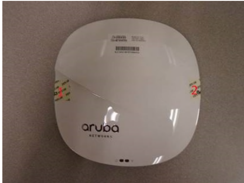
Figure 20 – Top View of AP-315 with TELs
