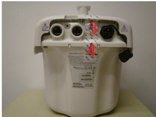
Figure 34 – Rear View of AP-275 with TELs
