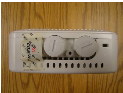
Figure 28 – End View of AP-228 with TELs
