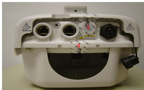
Figure 30 – Rear View of AP-274 with TELs
