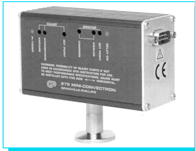
Figure 4-1 1 Setpoint MINI-CONVECTRON Front Panel Showing Indicators and Adjustments.
