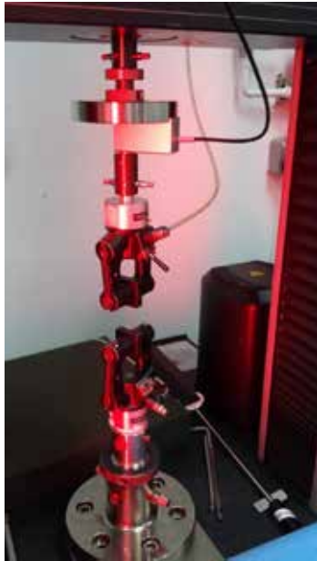
Figure 4.7 Instron 5569 Universal Testing System with pneumatic side-action grips and a mounted 20 x 5 x 0.53 mm h-PDMS strip. The overhead grip is attached to a 10N load cell. The strain was measured using a non-contact video extensometer at an extension rate of 1 \text{ mm min}^{-1} (strain rate of 0.05 \text{ min}^{-1} ).
