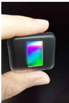
h-PDMS/PDMS composite test mould prior to cut-out
