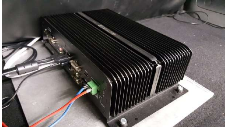
FIGURE 6.6: In-vehicle computer by Acrosser installed on the Smart-ED
