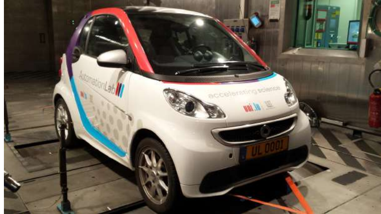
FIGURE 2.10: Smart-ED on the two-axle dynamometer test bench.
