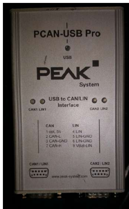
FIGURE 6.3: CAN adapter installed in Smart-ED
