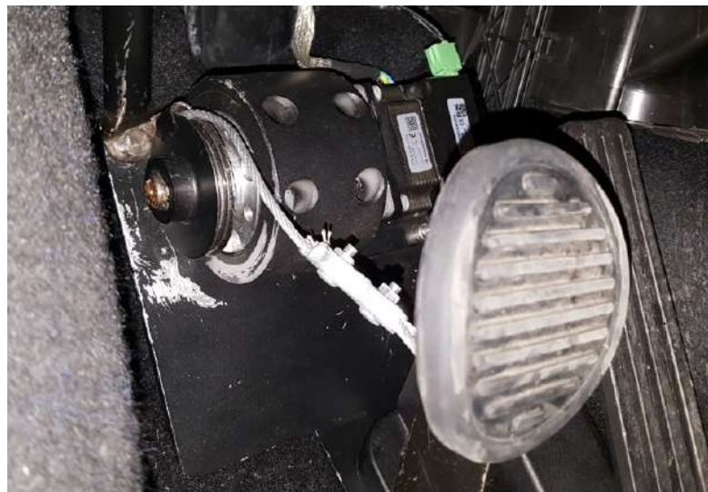
FIGURE 6.11: Brake pedal actuator installed on the Smart-ED
