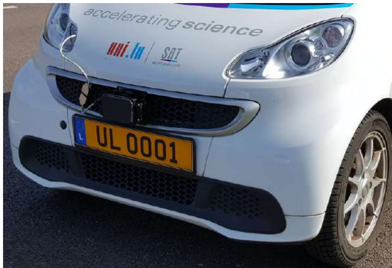
FIGURE 6.5: RADAR sensor installed on the Smart-ED
