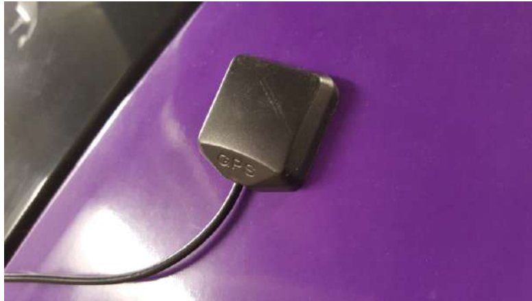
FIGURE 6.2: GPS sensor installed on the Smart-ED
