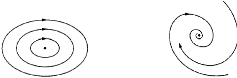
Fig 1.9 Schematic illustration of fixed point of a center (i) and a stable spiral (ii).
