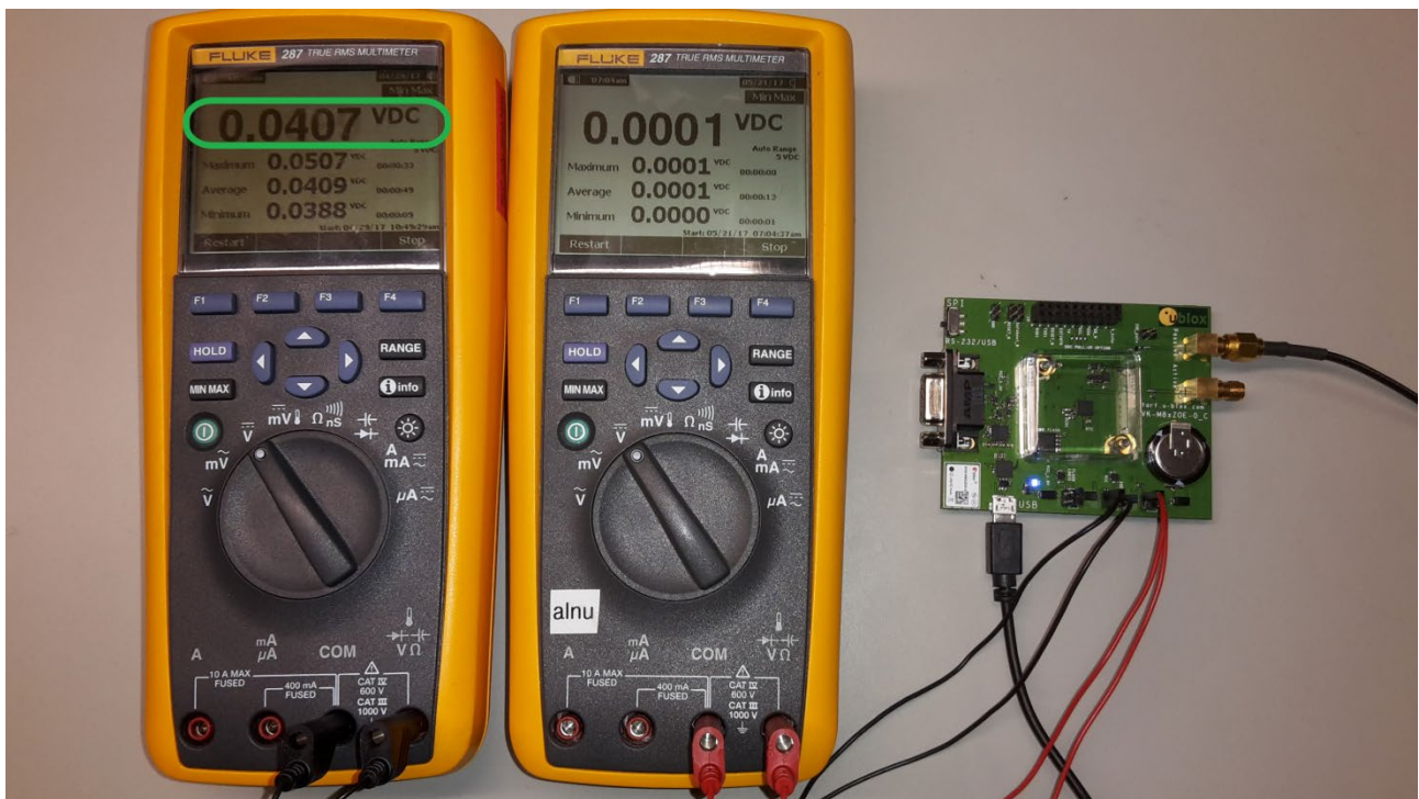
Figure 5: Setup to measure the VCC current consumption of ZOE-M8G on EVK-M8GZOE
