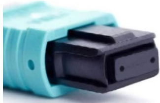
Transceivers have pins Optical connector has holes
