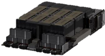
Internal DAC cabling Cedar-7-to-OSFP cages
