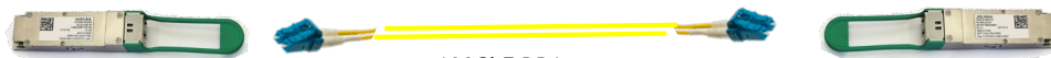
100GbE DR1 500m QSFP28 LC Single mode 4x25G-NRZ electrical -to- 1x100G-PAM4 optical MMS1V70-CM
