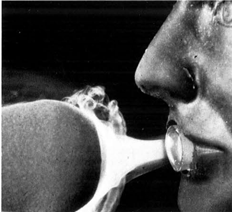
This laboratory test provides a visual representation of the air motion which occurs as a result of breath "pop." It is one of the many application tests used by Shure engineers in determining the optimum size and density of a microphone windscreen.
